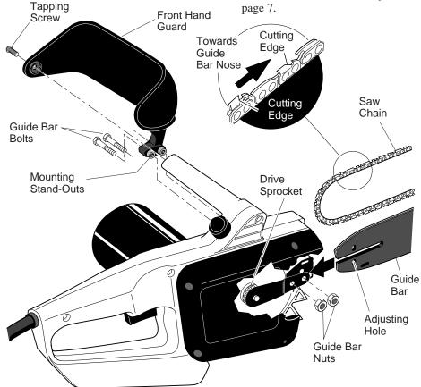
Figure 3 - Assembling Guide Bar, Chain, and Hand Guard
